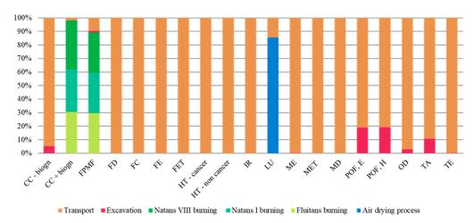
**Figure 11.** Percentage contribution of potential impacts to produce biomass by burning process for power generation.
