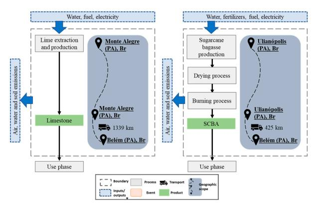
Figure 16. SCBA generation versus limestone extraction and production system boundaries.
