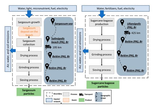
Figure 14. Sargassum versus Sugarcane bagasse particle production processes.
